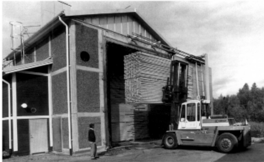
Workers place the last load of wet wood in Alent's kiln before closing the door. In about half of the traditional time, this lumber will be dry and ready to be used on any building project.
